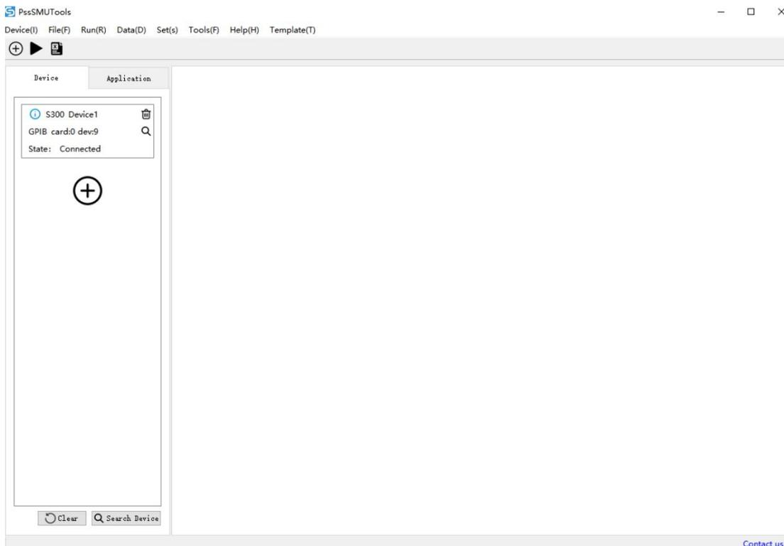
Figure 2-7 GPIB add new device
