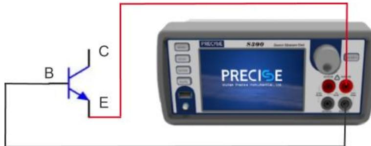
Figure 3-15  $V_{EBO}$  test circuit
