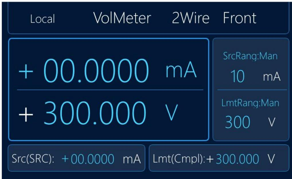
Figure 1-20 Voltmeter interface
