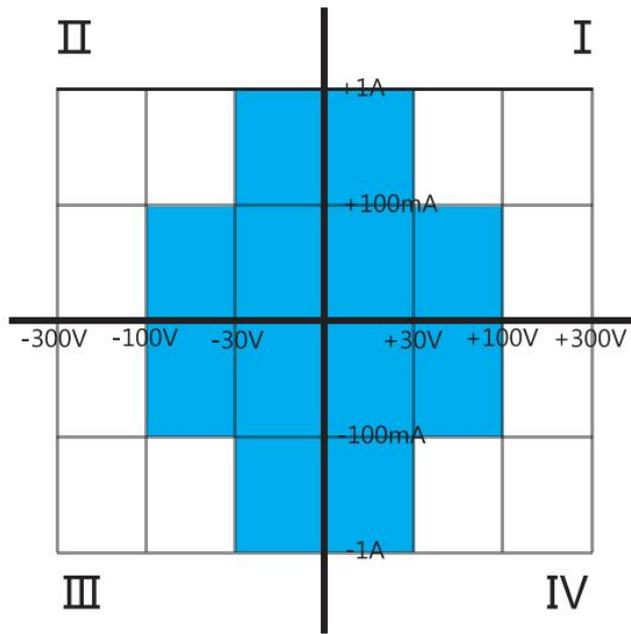
Figure 1-3 S200 four-quadrant working diagram
