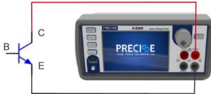
Figure 3-17  $V_{CEO}$  test circuit
