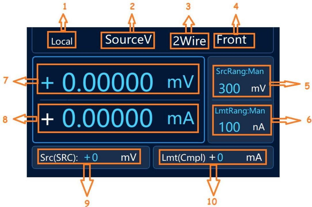
Figure 1-9 Measurement function window
