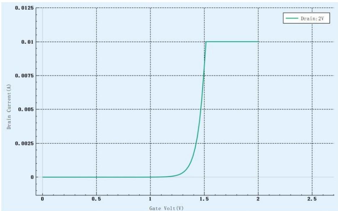
Figure 3-20 MOS input characteristic curve
