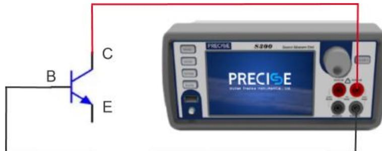
Figure 3-16  $V_{CBO}$  test circuit
