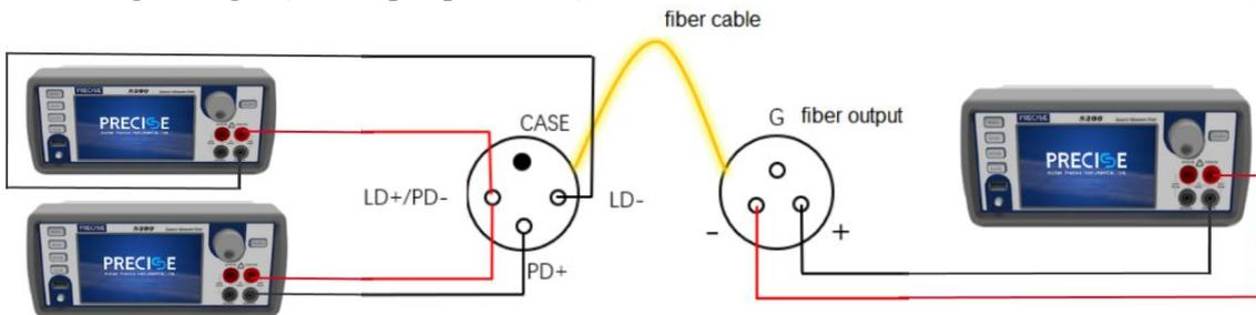
Figure 3-26 PIN test circuit
