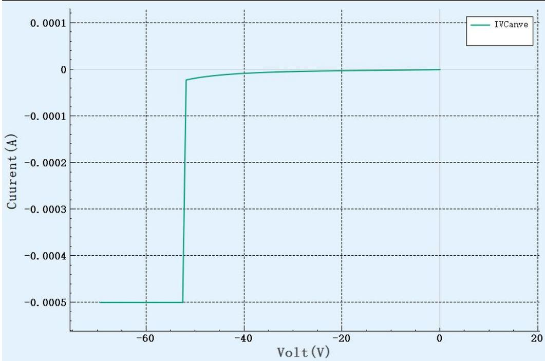
Figure 3-4 Diode reverse characteristic curve
