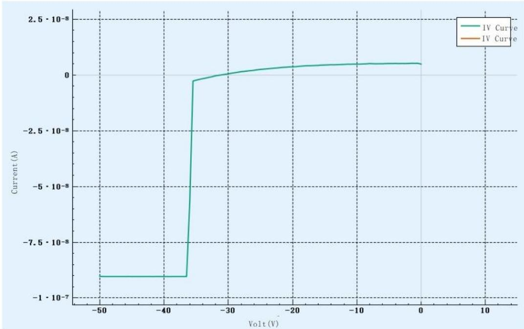
Figure 3-25 APD characteristic curve
