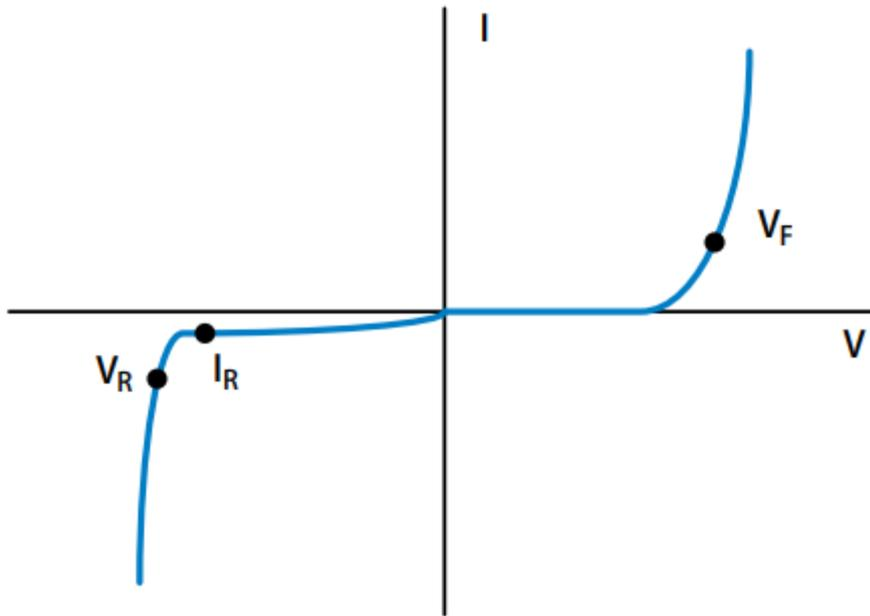
Figure 3-1 Diode typical I-V curve
