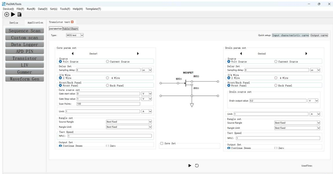
Figure 2-16 MOSFET test interface
