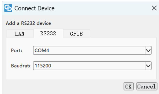
Figure 2-4 PC serial port connection settings
