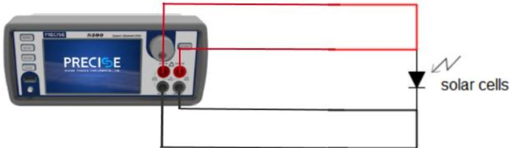
Figure 3-27 Solar cells test circuit
