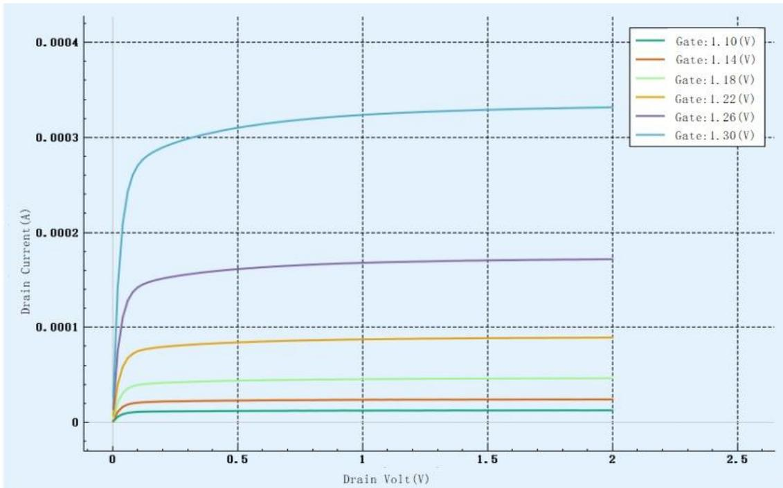
Figure 3-21 MOS output characteristic curve
