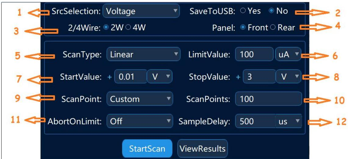
Figure 1-18 Scanning function window
