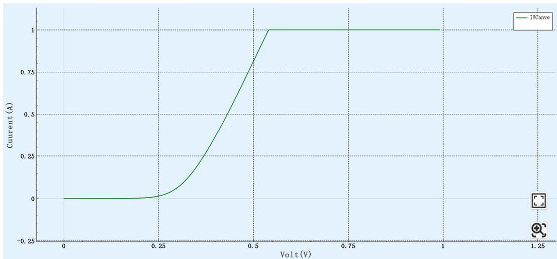
Figure 3-3 Diode forward characteristic curve
