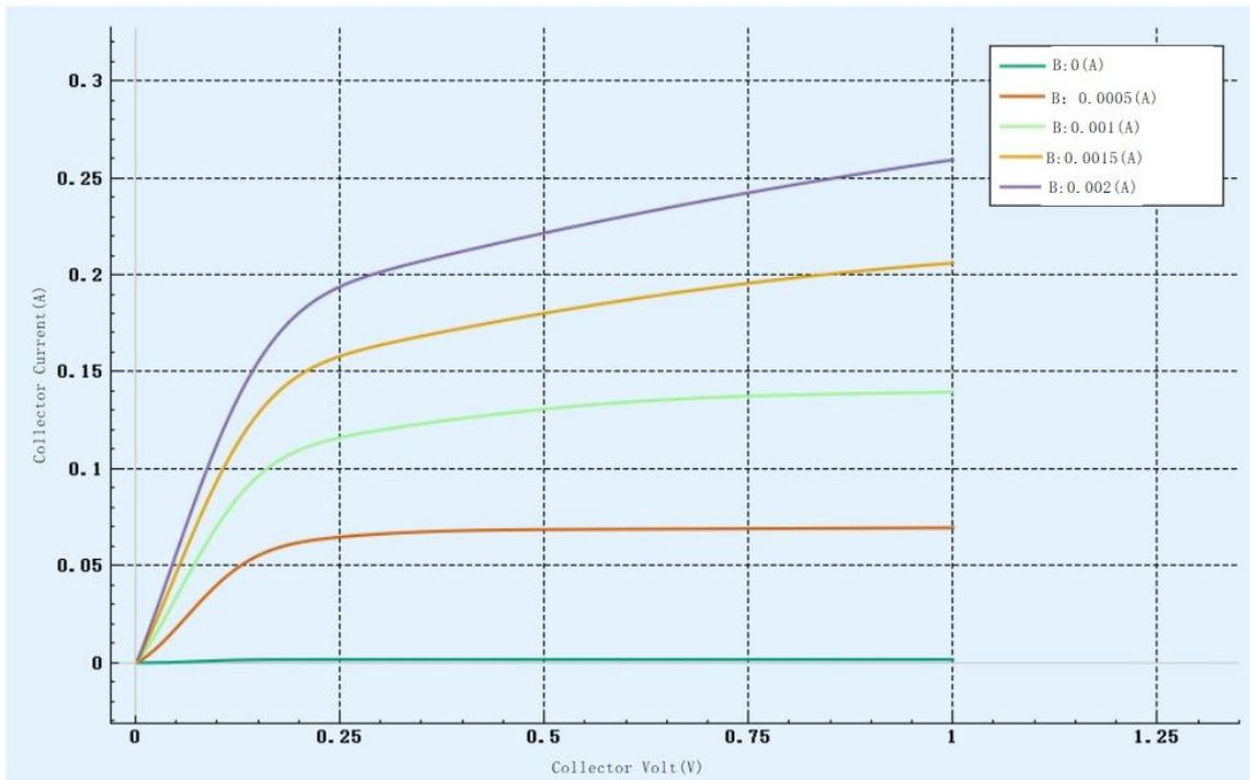
Figure 3-11 Transistor output characteristic curve
