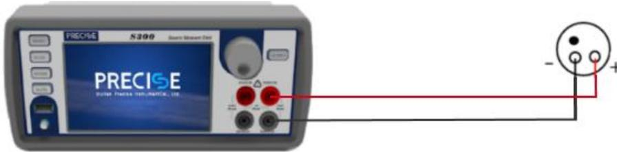
Figure 3-24 APD test circuit
