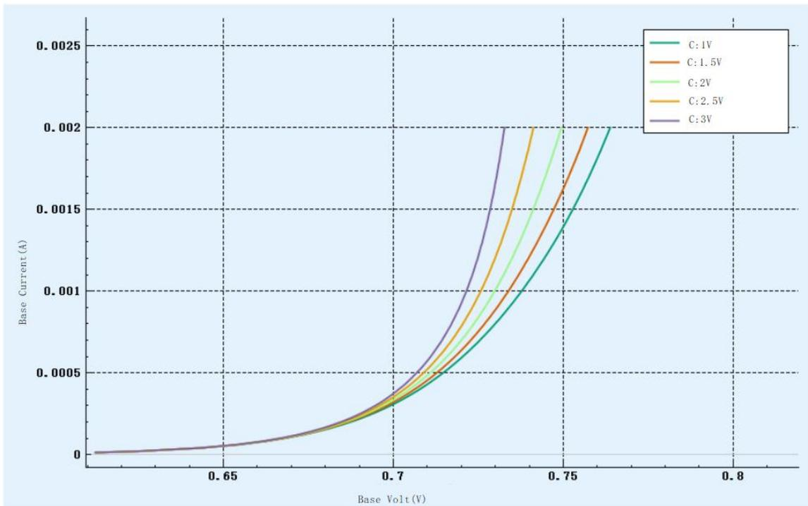
Figure 3-10 Transistor input characteristic curve
