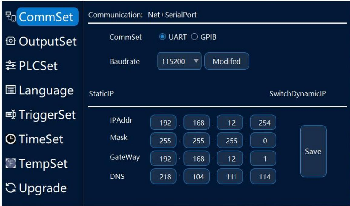
Figure 1-11 Communication configuration
