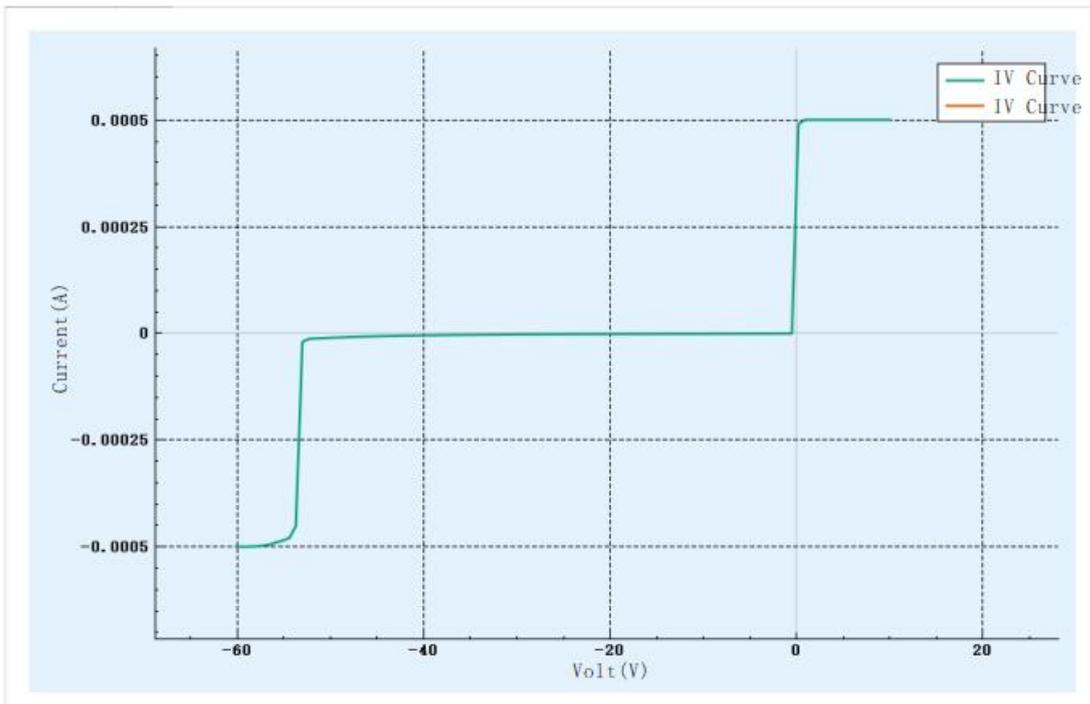
Figure 3-7 Complete diode characteristic curve
