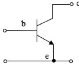
Figure 3-8 Common Emitter Connection
