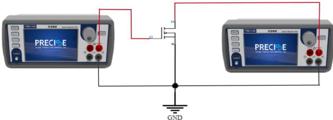
Figure 3-19 MOSFET test circuit
