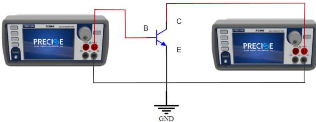
Figure 3-9 Triode test circuit
