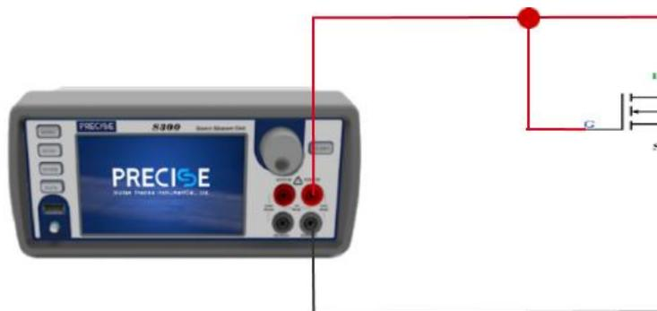
Figure 3-22  $V_{GS(th)}$  test circuit
