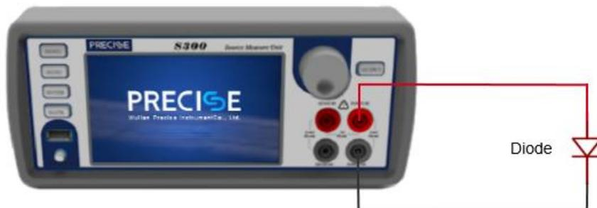
Figure 3-2 Diode test circuit diagram
