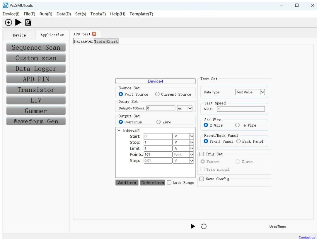
Figure 2-15 APD test module interface
