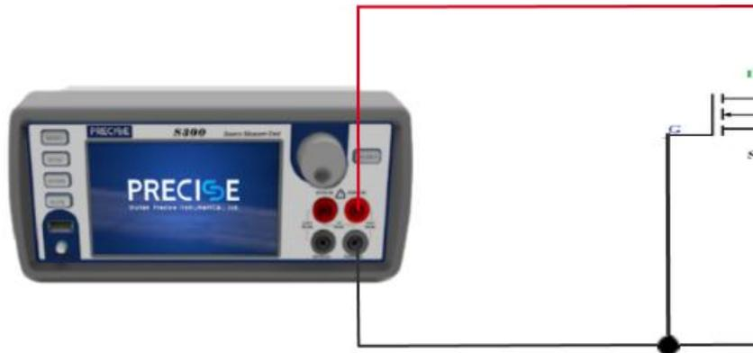
Figure 3-23  $V_{DS}$  test circuit
