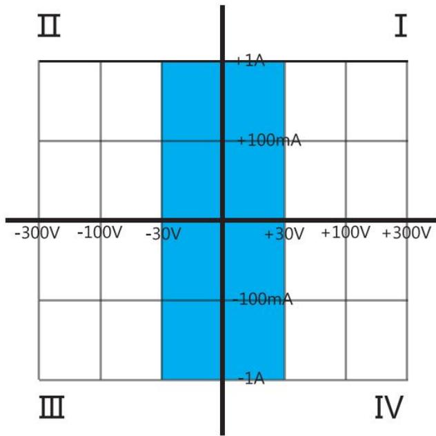
Figure 1-2 S100 four-quadrant working diagram
