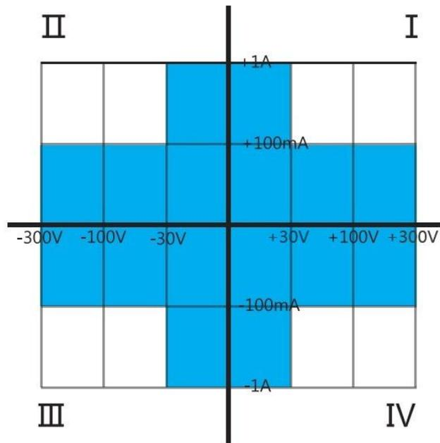
Figure 1-4 S300 four-quadrant working diagram
