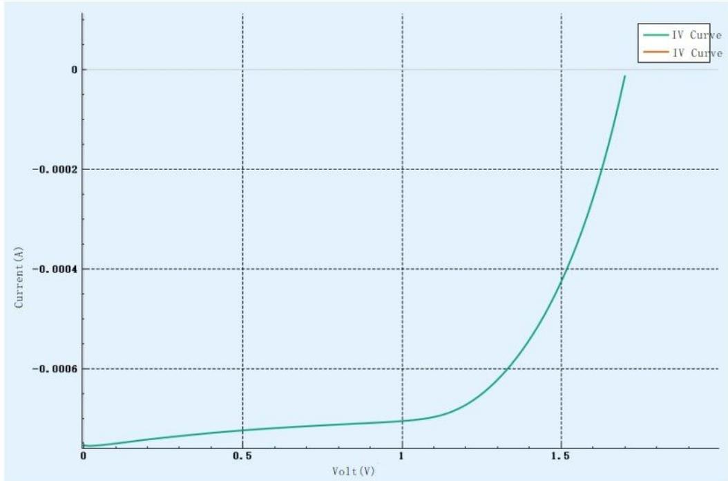
Figure 3-28 Solar cells scanning curve
