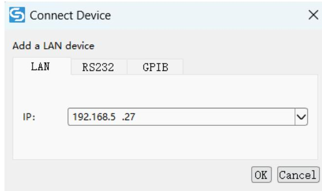
Figure 2-2 PC network port connection settings
